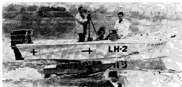
Fig. 3 LOWTS testing hydro-ski assault craft.
